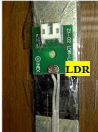
Figure 2 Illuminance sensor developed from LDR
