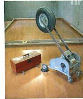
Floor impact sound test (Acoustic test)
