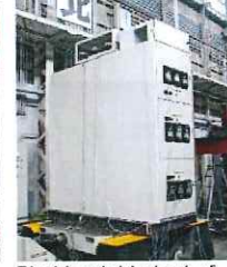
Shaking table test of electric equipment
