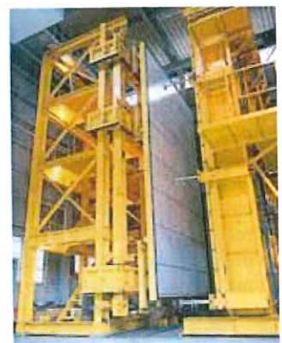
Test on Deformation Capacity of exterior wall (Aerodynamic test)
