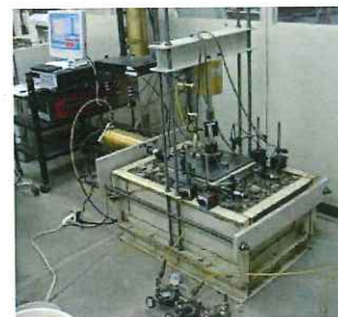
Friction test of drainage mat for retaining wall
