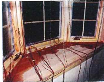
Dew condensation test (Thermal test)
