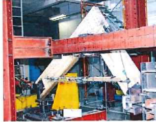
Test of timber frame joint
