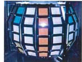
Light-exposure test of internal finishing materials (Enclosed carbon-arc type)
