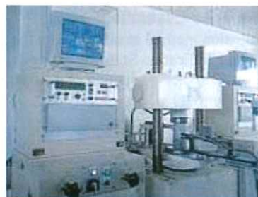
Automatic compression test system for concrete cylinder specimens.
