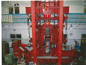
Testing setup for simulated earthquake loading on columns or beams
