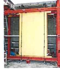
Shear test of timber wall
