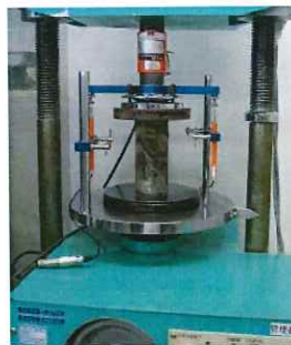
Unconfined Compression test of improved soil
