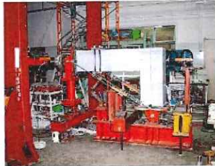
Test of R/C corner joint
